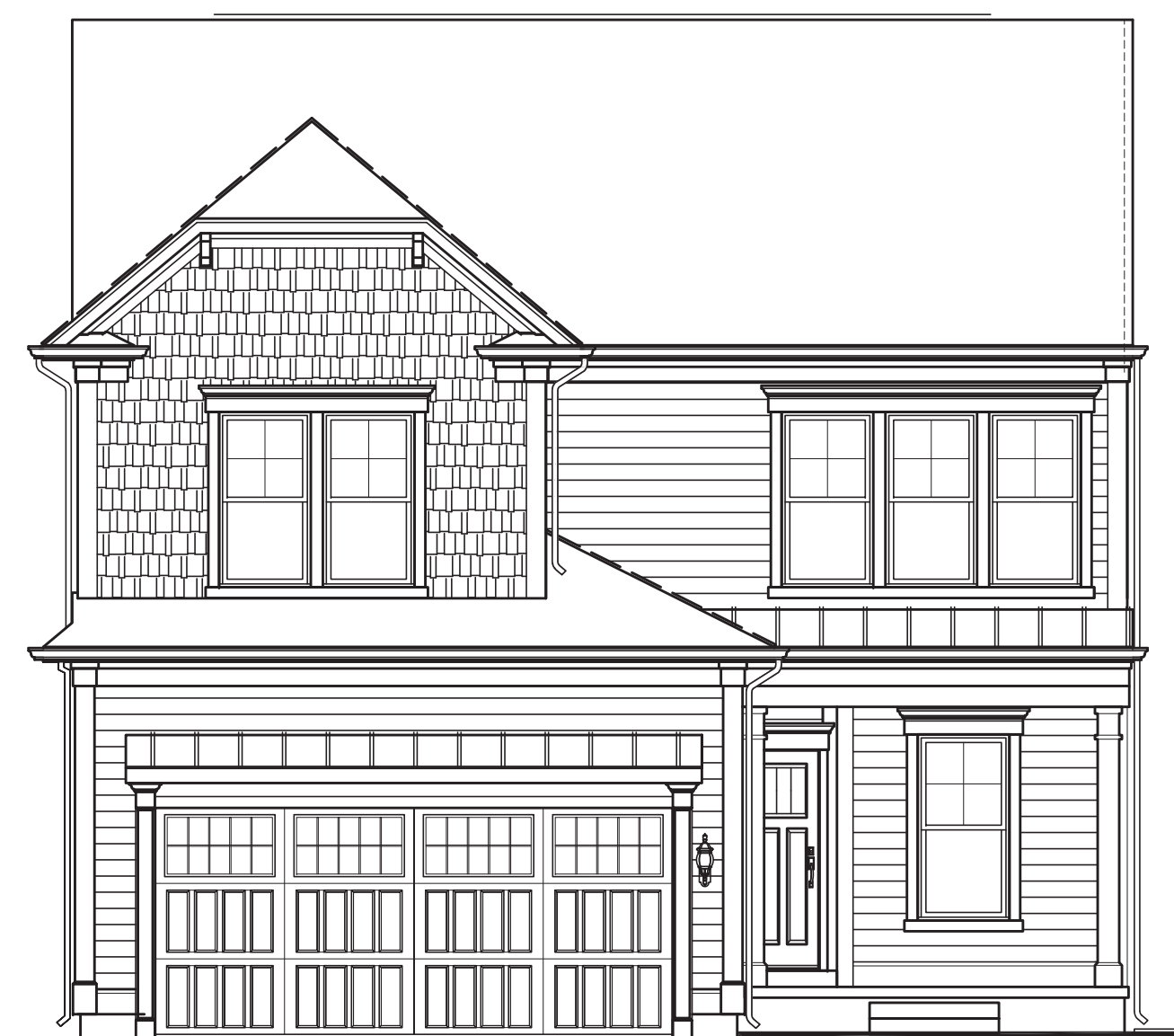
FRONT ELEVATION # 1 SHOWN WITH OPTIONAL WINDOWS AT GARAGE DOOR 3/16"=1'-0"
