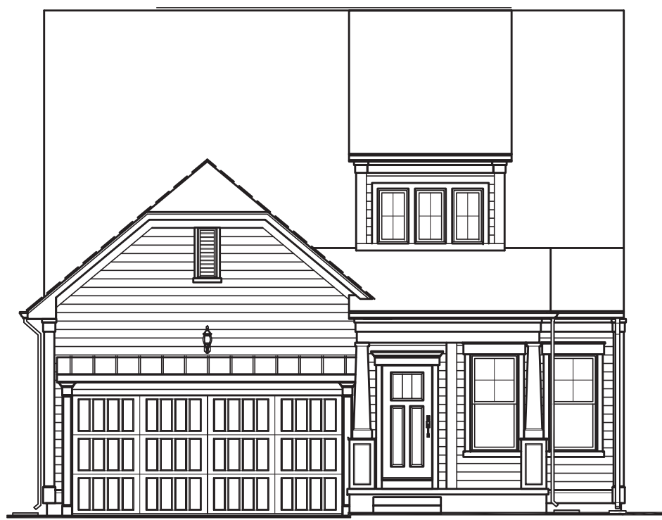
FRONT ELEVATION # 3 SHOWN WITH OPTIONAL WINDOWS AT GARAGE DOOR 1/8"=1'-0"
