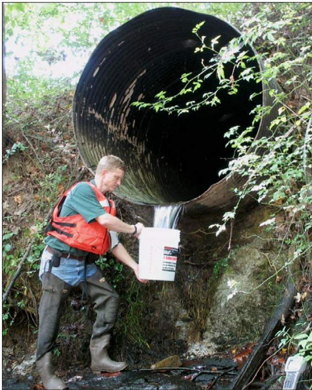
Figure 5. Measurement of streamflow and water quality in a small watershed with a high density of septic systems, Gwinnett County, Georgia, October 16, 2007.
