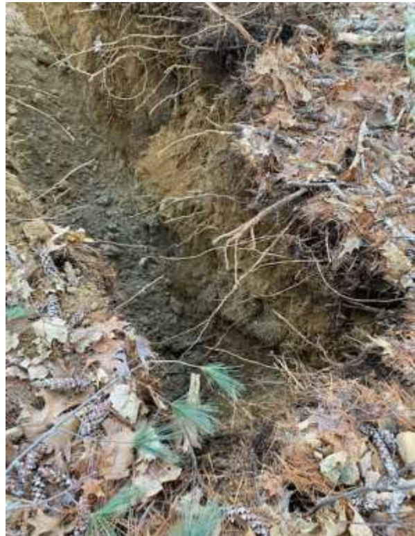
Test pit exhibiting a profile with 2 general categories of soil: sandier material (brown hue) near the surface and glacial till (grey hue) deeper.
