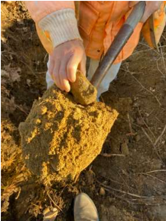
Soil collected for grain size analysis (sieve analysis). Corresponds to the upper layer in the photo to the right (note color). Sand, loamy sand, and/or sandy loam.
