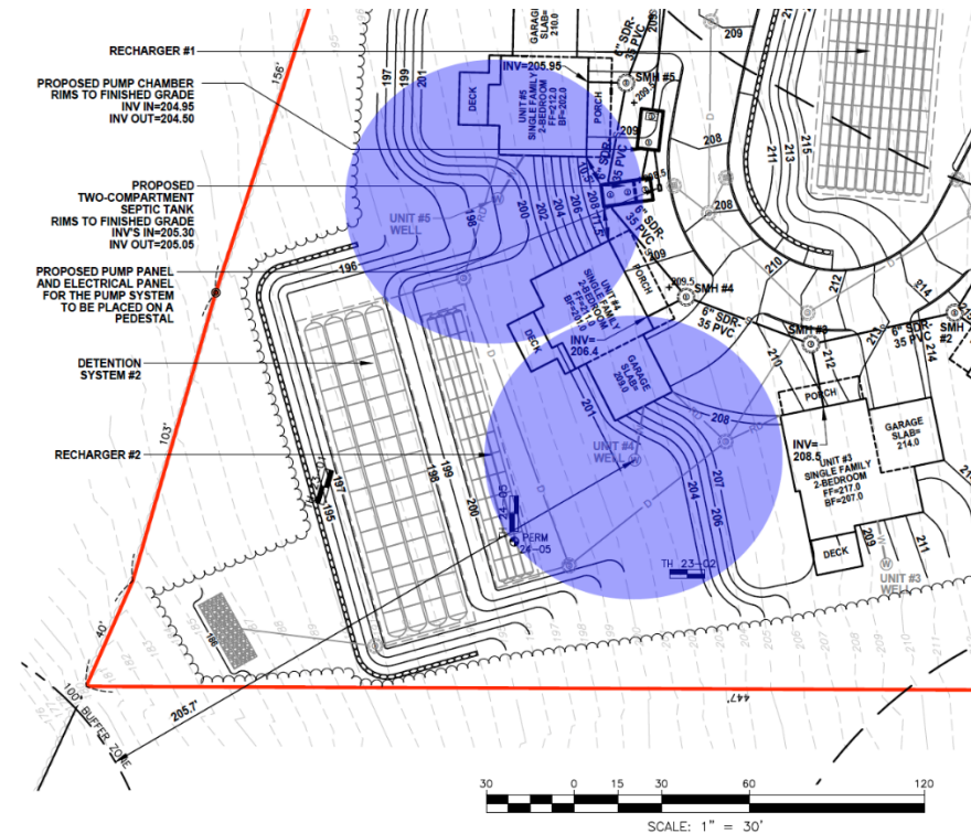
Figure 7 – Recharger 2 Infiltration System and 100-foot required buffers to private wells
